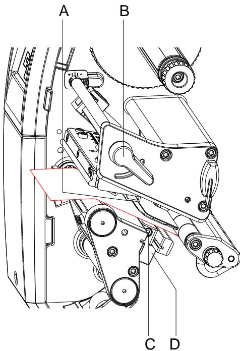
The label sensor can be shifted perpendicular to the direction of paper flow for adaptation to the label medium. The sensor unit (A) of the label sensor is visible from the front through the print unit and is marked with an indentation in the label sensor retainer.
