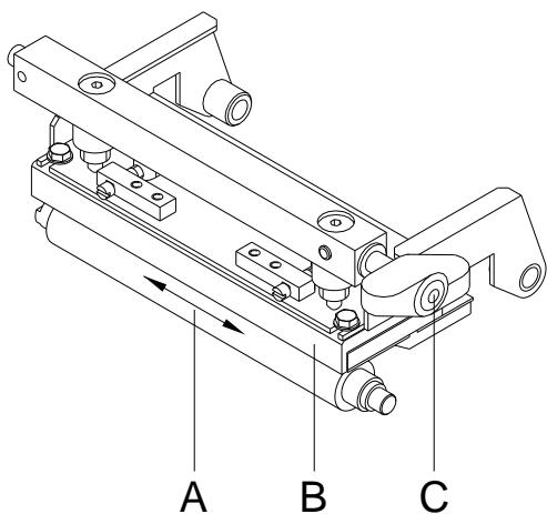
A soiled pressure roller can lead to a reduced print quality and can affect the transport of material.
